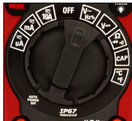
Range selector illuminates to allow for easy selection in dark areas
