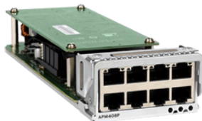
8x10GBASE-T PoE+ Port Card - 100M/1G/2.5G/5G/10G (APM408P)
